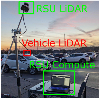
Figure 13: VRF deployment setup.
